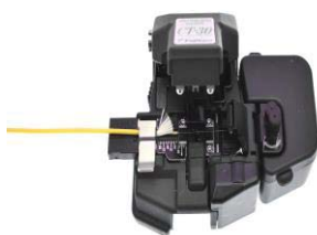
Figure 77: Cliver la fibre
