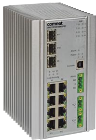
CNGE11FX3TX8MSPOE[HO] 11-Port All-Gigabit Managed Switch with 30 W PoE+ / 60 W Universal PoE 3 Gigabit SFP Ports (FX) 8 Gigabit Copper Ports (TX) with PoE
